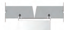
TBV 03 - Bevelled Joint 3mm Gap
