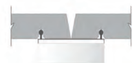
TBV 03 - Bevelled Joint 3mm Gap
