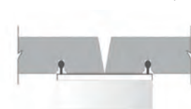
TBV 03 - Bevelled Joint 3mm Gap
